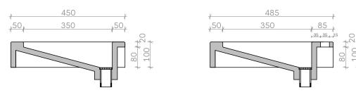
All product sizes are in millimeters and have an informative character. The producer reserves the right to amend the technical specification at any time without previous warning. This sink does not have an overflow hole. Valid from: 22.08.2017
